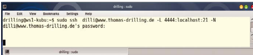
Figure 6: The -N parameter prevents a shell from being launched on the remote system through local port forwarding.
