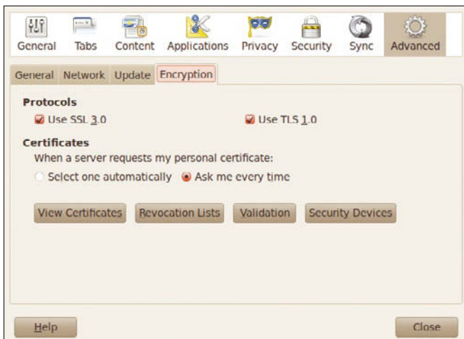
Figure 2: Especially while setting up the server, it is helpful to have Firefox prompt for the certificate every time.
